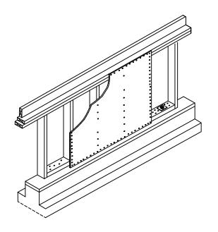
Plywood is then stapled to the blocks and this attaches the plywood to the the mudsill.
