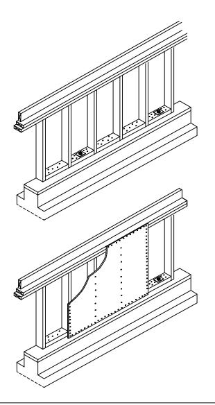
2"x4" blocks are nailed into the mudsill between studs.
