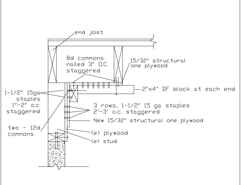
Shear Wall Repait missing topplate, plywood to next joist
