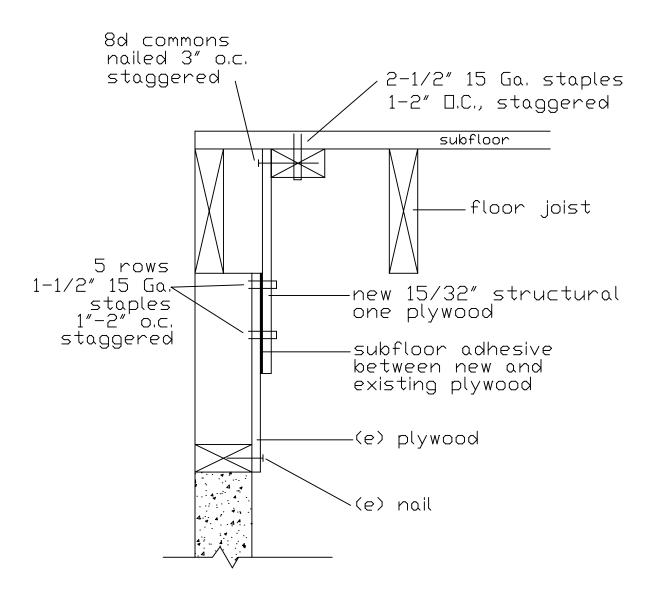
Shear Wall Repair staple 2 by to subfloor
