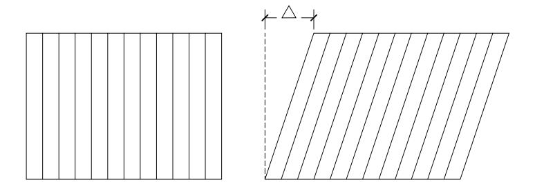
Deformation of a Rectangular Plywood Shearwall
