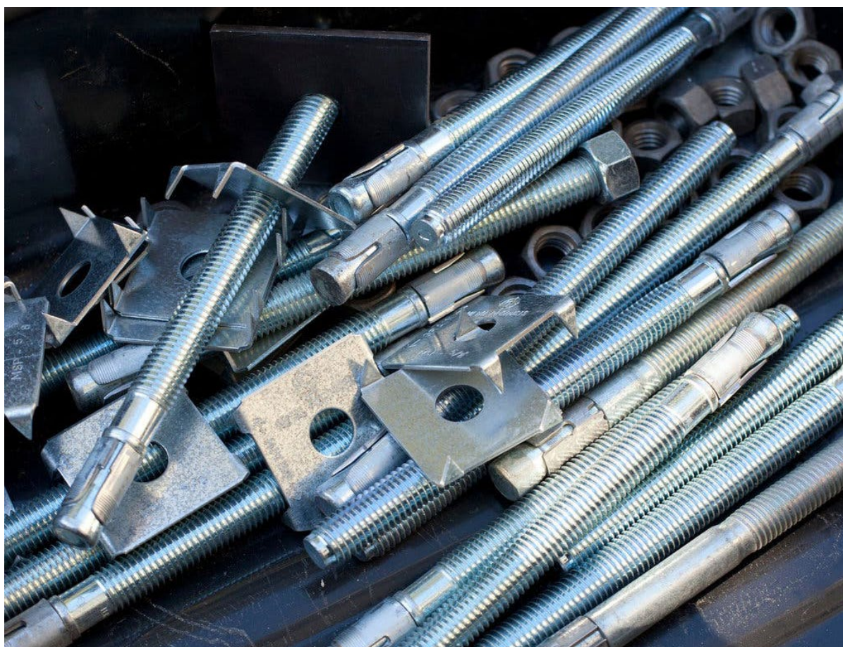
Anchor bolts used in the project. Peter DaSilva for The Bay Citizen
