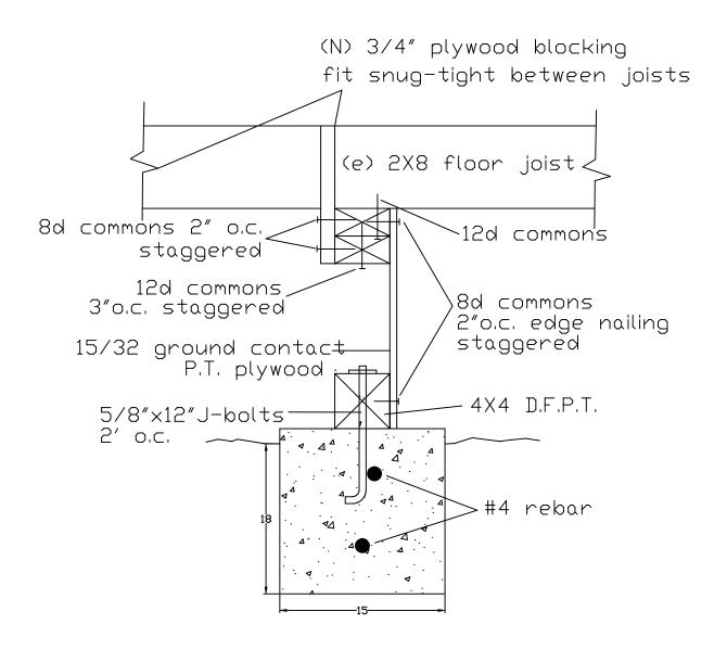
New Footing and Shear Wall with plywood blocking (Two Story Building)
