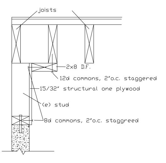
Used when no topplate is present and distance between end joist and first joist makes installing a topplate impossible.
