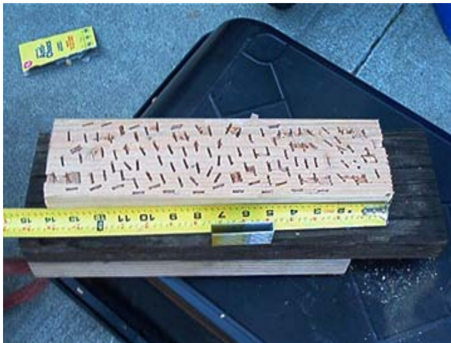
This photo shows a 14-inch block with 114 2-1/2 inch staples. Notice no splitting of the block.
