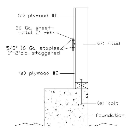
For new walls or when the contractor neglected to install horizonal 2x4 blocks between plywood panels. See APA Techincal Note #N370C, May 1997.
