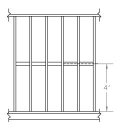
Install flat 2by blocks in stud bays so that the blocks are centerd at the plywood edge joint.
