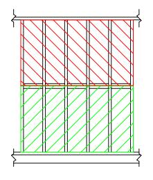
Place the top sheet of plywood on the bottom sheet. Staple it to the blocks. Pop a chalk line if you need to to make sure you hit the blocks.
