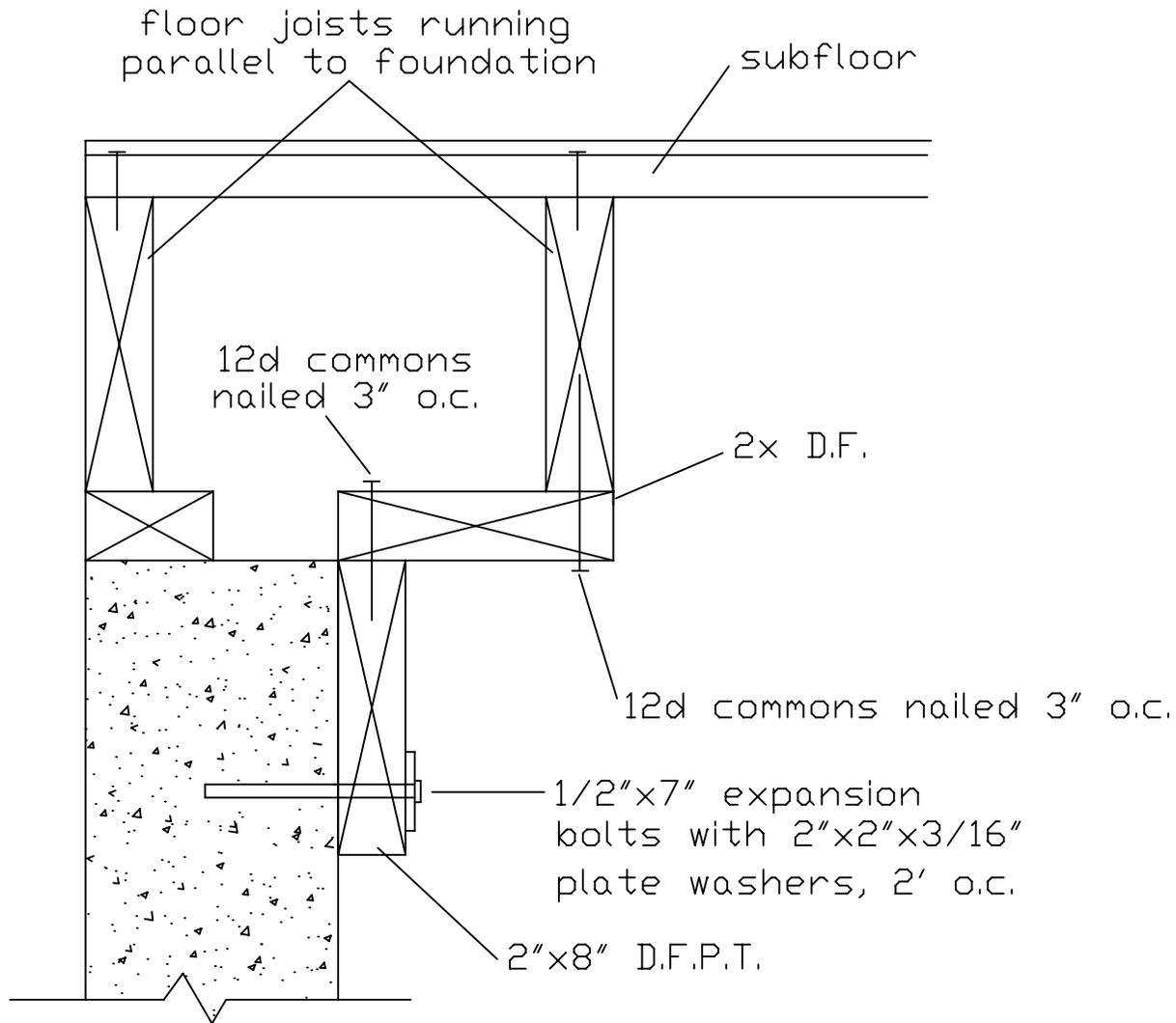
Bolting of floor to foundation when gap between edge of concrete and edge of mudsill exceeds 2-1/2" or when no mudsill is present.
