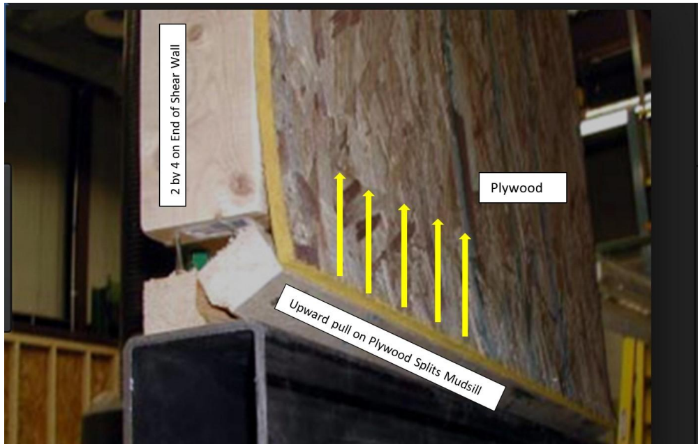
Photo: Cross-grain bending damage to mudsill in a testing laboratory.
