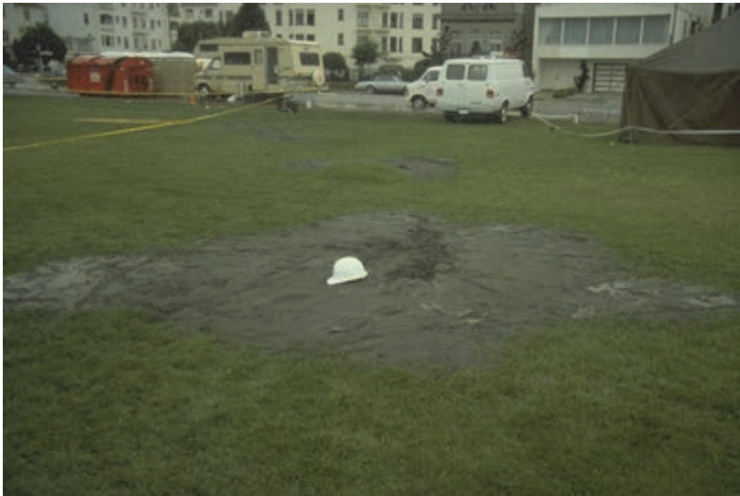
Figure 5-12 Sand ejecta after liquefaction of hydraulic fill from the 1989 Loma Prieta, California earthquake (photo credit: NISEE).
