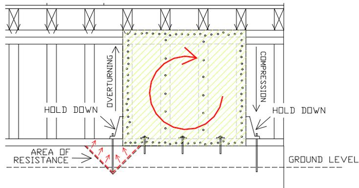
Hold down bolts will pull up on the concrete they are attached to. For this reason the bolts should be installed as deep as possible into the existing concrete and epoxied into place according to the manufacturer's instructions.
