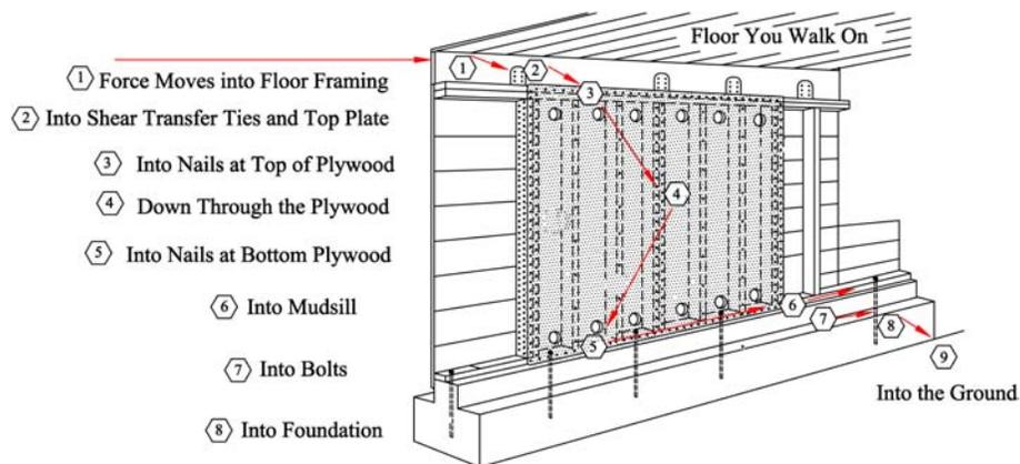
Load Path of Earthquake Forces
