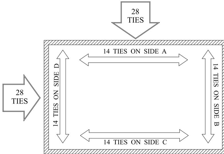
**Diagram 11:** Required number of shear transfer ties
