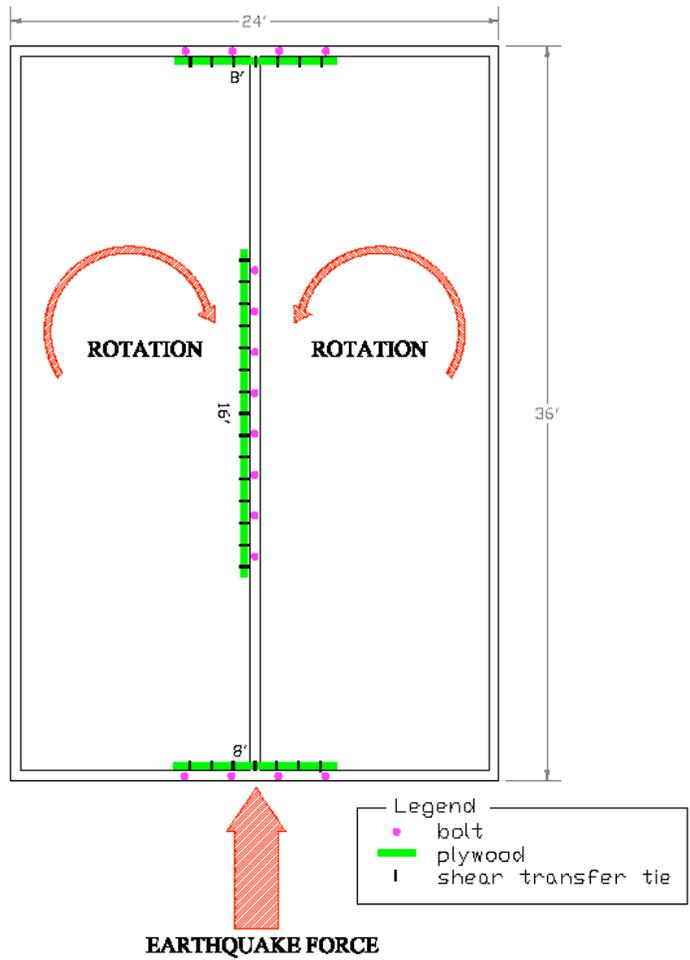
If one side of the house has obstructions that prevent access to this cripple wall, and it does not possess a center foundation, a house can be retrofitted by bracing the cripple walls on the opposing side only. This approach uses the code citation mentioned above.
