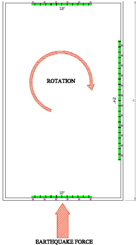
Houses with a living area above a garage have a serious problem because a shear wall cannot be built under the edge of the floor above the garage door opening without obstructing access to the garage. The posts and short segments of wall on either sides of the garage door opening will tend to tip over in an earthquake. The Building Code requires that in order to be effective these walls be 4 feet wide.
