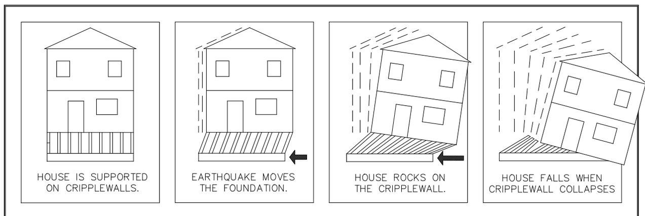
**Figure. 1:** Damage to house due to lack of cripple-wall bracing
