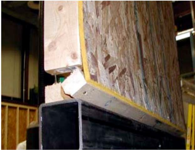
Cross grain-bending failure in test shear wall
