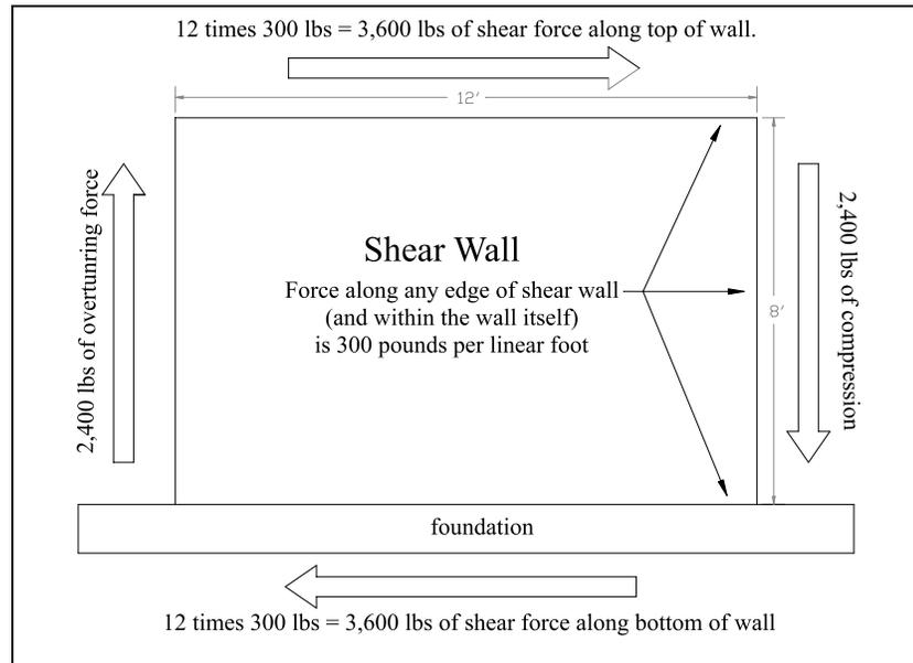
In this example the shear wall absorbs 300 pounds of lateral force for each linear foot of plywood. Thus the top and bottom are 12 feet long and thus must resist 3,600 pounds each; the 8 foot tall left and right sides, 2,400 pounds each. A shear wall is designed to resist this force on all sides of wall. Notice how the left side of the shear wall is being pulled up and the right side pushed down. Hardware that resists this lifting up or overturning force is called a hold down.
