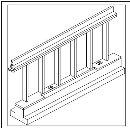
This illustration shows the mudsill cut flush with the rest of the 2 by 4 wall framing.
