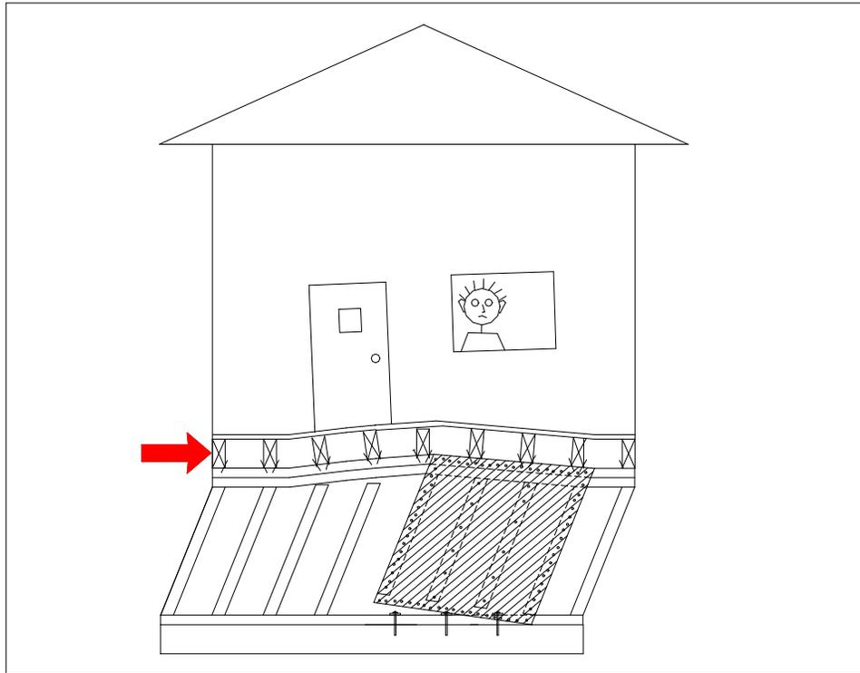
Here is an example of a shear wall overturning. This drawing is exaggerated in order to illustrate what happens. Most of the damage to the shear wall occurs where the plywood lifts up and away from the mudsill. The house will also sustain a significant amount of damage. Below is a close up illustrating tearing of the plywood at the mudsill. Once this happens the shear wall cannot longer transfer shear forces into the bolts.
