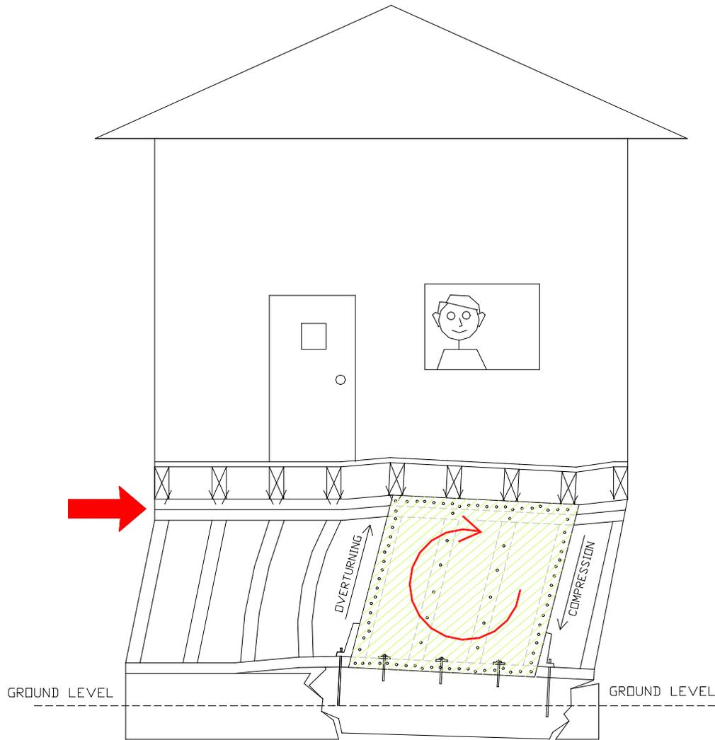
Sometimes the overturning forces are so great that an un-reinforced concrete foundation breaks, or an improperly reinforced foundation deforms. This can lead to a lot of movement of the floor that results in significant damage to the structure.
