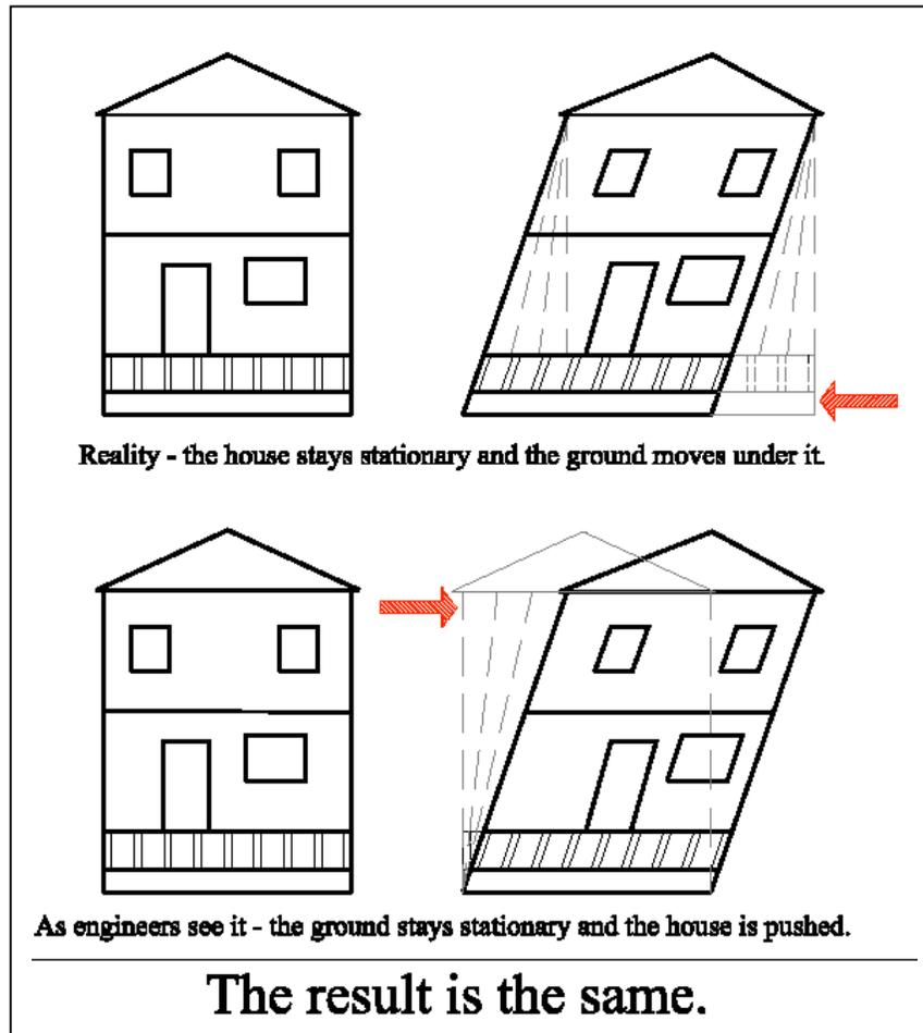
The purpose of retrofitting is to keep the house on the foundation when pushed on as shown above. This is done by inverting un-braced cripple walls into earthquake resistant shear walls. Retrofit shear walls consist of three different retrofit components:
