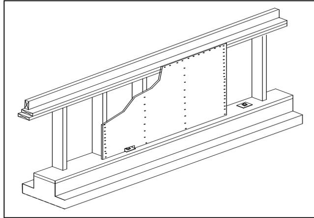
The mudsill is wider than the 2 by 4 upright studs and top plate. This makes it impossible to nail the plywood to the bolted mudsill without framing modifications.
