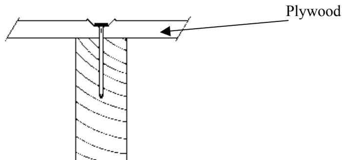
If the nails are spaced close together re-nailing the plywood may cause the wall framing to split. I recommend repairing the shear wall according to Technical Note TT-012 American Plywood Association available on the internet. This option will allow you to repair the plywood to framing connection rather than remove and replace it.
