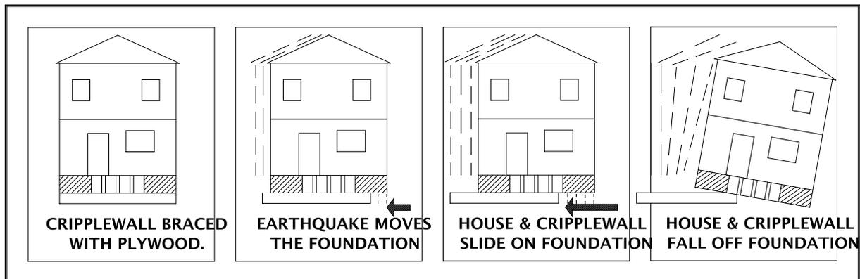
**Figure 2:** Failure caused by lack of foundation bolts
