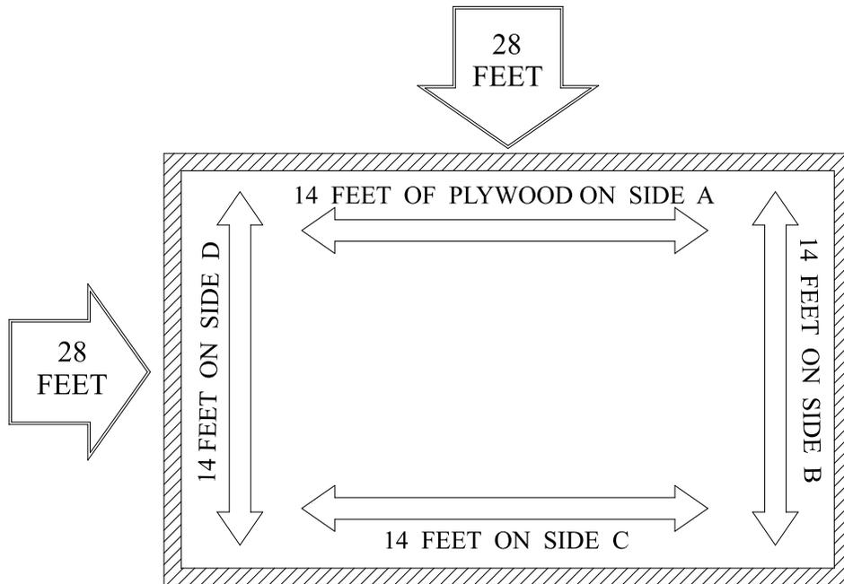
**Diagram 10:** Required linear footage of plywood
