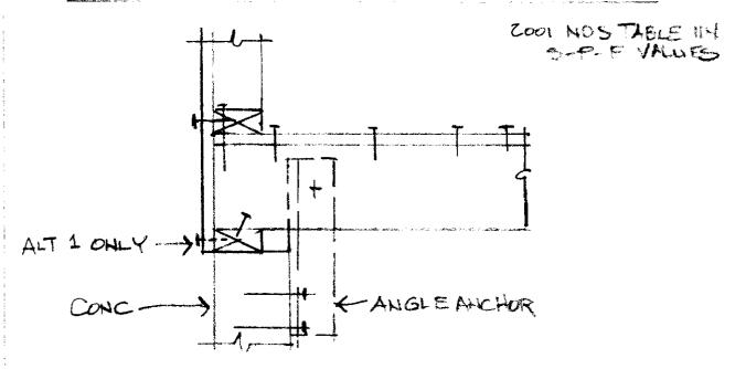
ALT 1 - EXT SHEATHING TRANSFERS ALT 2 - EXT SHEATHING LOAD TO SILL PLATE
